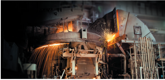
Electric arc furnace at a Nucor steel plant
