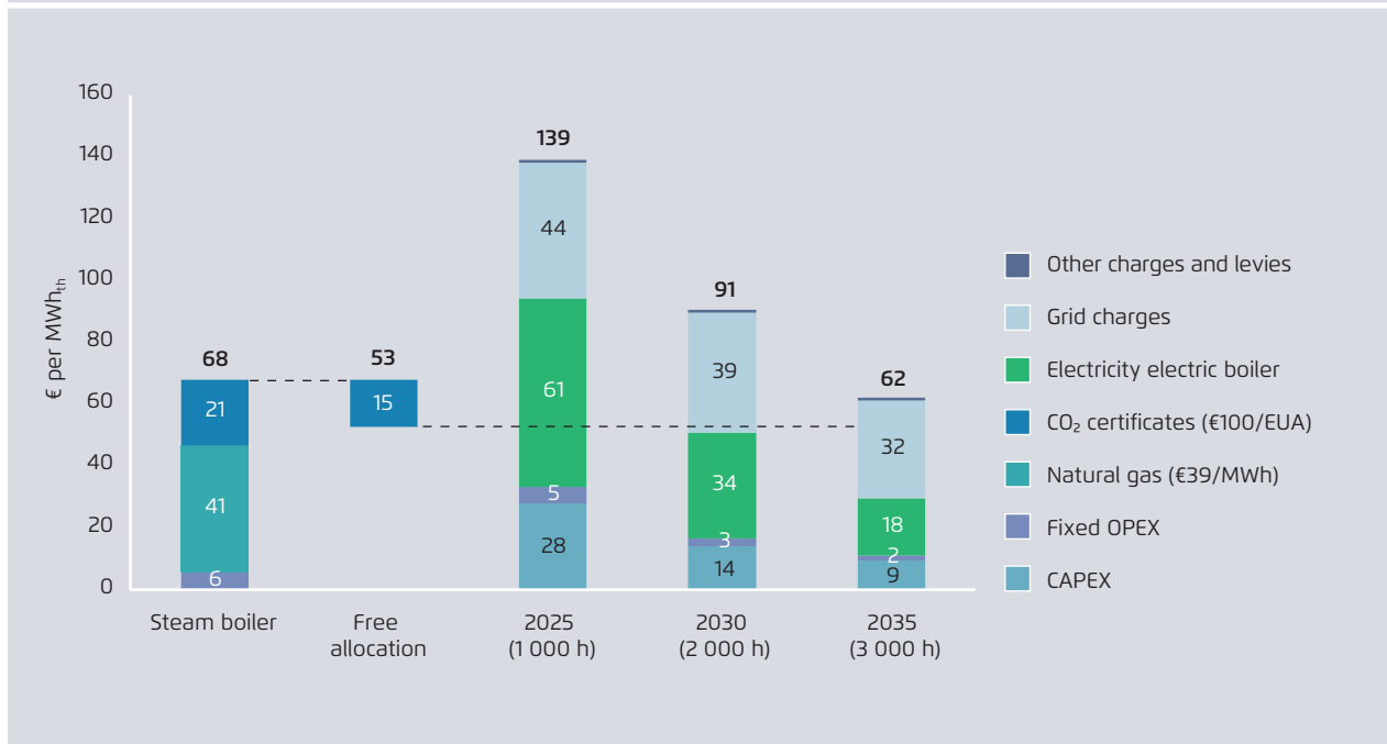
Average costs for operating an electric boiler compared to a gas-fired steam boiler for the years 2025, 2030 and 2035 with increasing full-load hours
