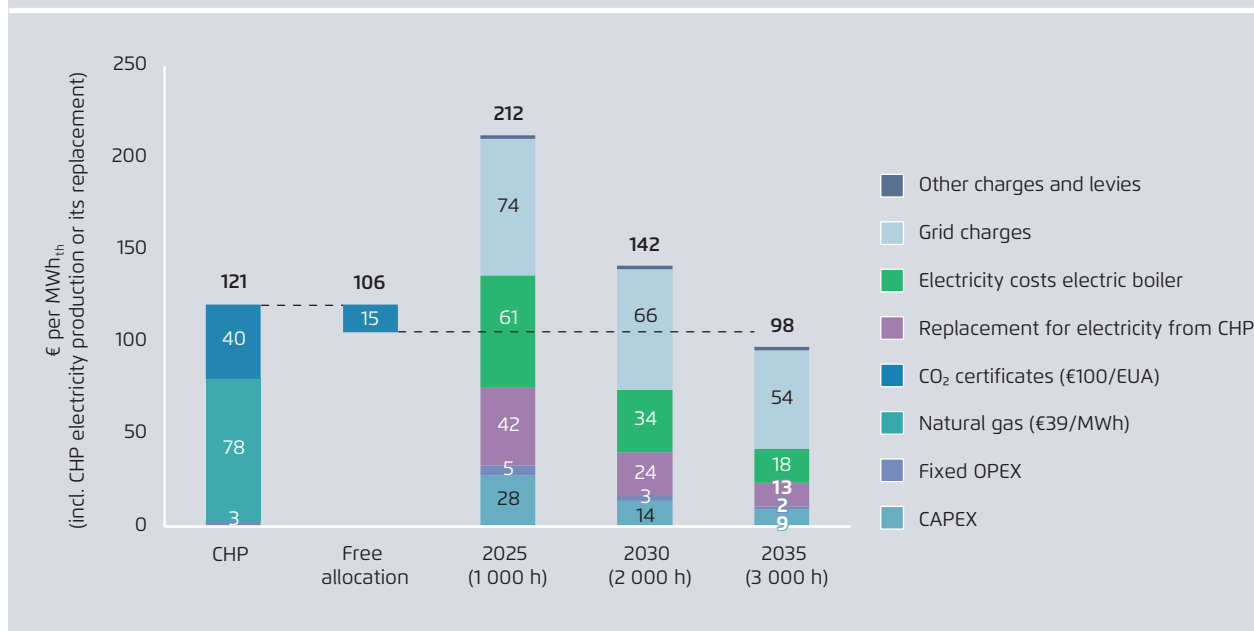
Average costs for the operation of an electric boiler in comparison to a gas-fired CHP system for the years 2025, 2030 and 2035 with increasing full-load hours
