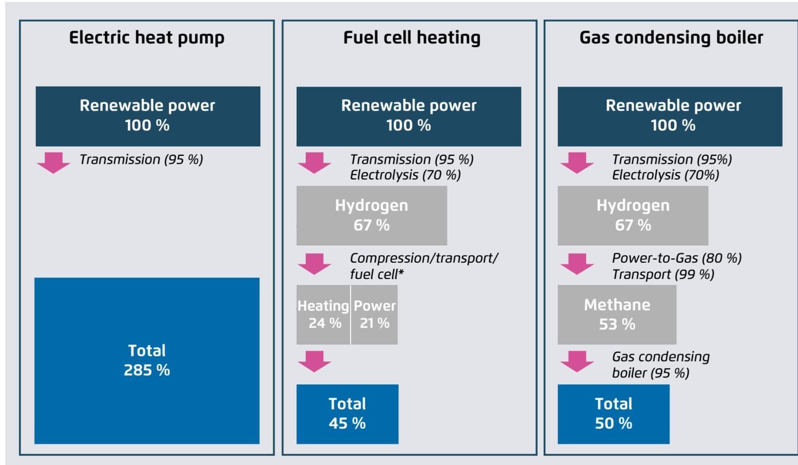
→ The electric **heat pump** withdraws more energy from the environment (air, soil or water) than required in terms of operational power, which is why it can have an efficiency rating over 100 %.
