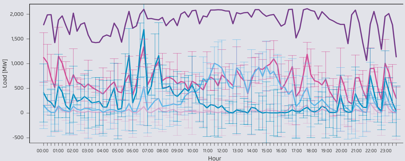
Cluster analysis of all of the year's diurnal variations (light pink, pink, blue, light blue) and quarter-hour balancing energy activation maximum throughout the year in magenta
