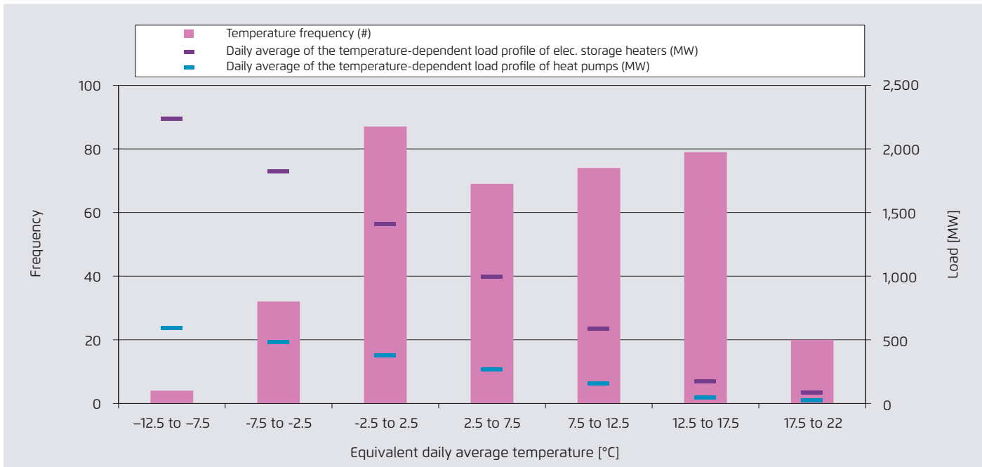
Frequency of the temperature ranges in southern Germany based on valid test reference years and the corresponding load profile averages of electric storage heaters and heat pumps
