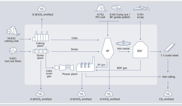
Agora Industry and Wuppertal Institute (2024). Note: Process diagram shows emissions from major point sources only. Additional emissions from distributed sources amount to  $0.08 \text{ tCO}_2/\text{t}$  of crude steel.
