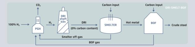
Agora Industry and Wuppertal Institute (2024). Note: Simplified carbon flow in the  $H_2$ -DRI-EAF and  $H_2$ -DRI-SMELT-BOF routes, assuming the DRI is produced with 100%  $H_2$ . PGH = process gas heater
