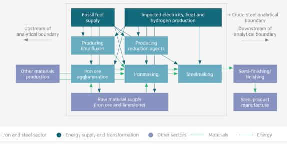
IEA (2022) Notes: "Other materials production" refers to the production of material inputs to the iron and steel sector besides iron ore and limestone, including electrodes, alloying elements and refractory linings.
